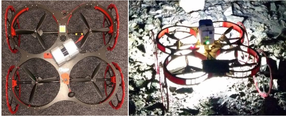
Figure 8 V-SCAN3D mounted on the Tilt Ranger drone developed by Inkonova, Sweden
